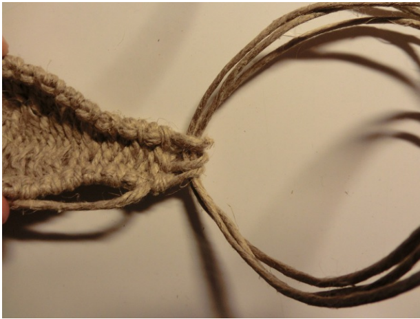
Figure 34: For the retention and release cord we will do a six strand round braid. Cut six strings of 4 times the wanted length of the retention and release cord. Loop three strings into the standing loops of one flap and center them.
